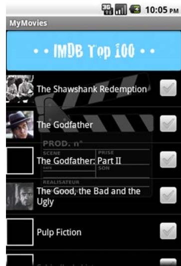
Figure 6.9 We'll simplify the code from the previous technique by using AsyncTask's built-in user interface hooks. We'll also added a placeholder image for those images that have yet to be loaded.
