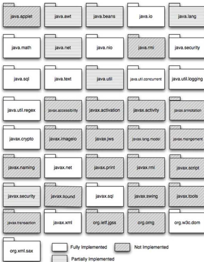
Figure 1.7 A graphical representation of the top-level packages in the standard Java runtime and their status in the Android runtime
