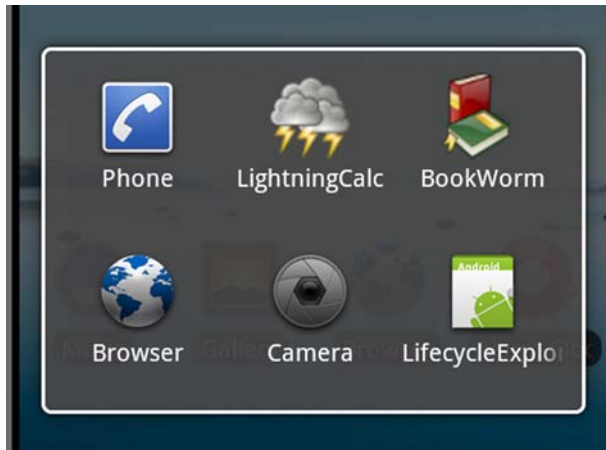
Figure 3.12 The recent tasks switcher shows the tasks a user can navigate back to displayed using the root activity's icon.
