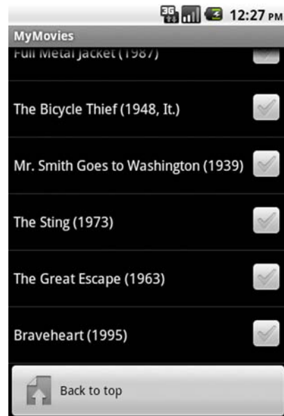
Figure 4.8 We added a button that returns us to the top of the list using a list footer view. The button icon can be set using the setCompoundDrawableWithIntrinsicBounds method.
