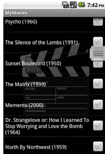
Figure 4.9 The MyMovies title screen after some styling has been applied. Note how we included a transparent background image and added a fast scrolling handle.
