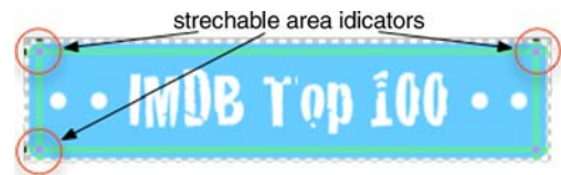
Figure 4.14 MyMovies title image defined as a nine-patch drawable; the corners demarcated by the black lines will be used for scaling (no padding has been defined).
