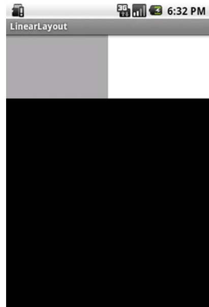
Figure 4.5 Two views arranged using LinearLayout . You can see how both views are sized to take the same amount of space and are aligned horizontally.
