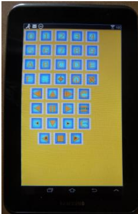
Screenshot of an Android Tablet that can be used as a Remote Control for Cinelerra Recording and Playback.
